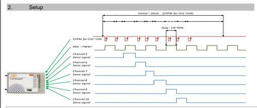
Warning: Servos are not to be plugged into Channel CPPM and Channel RSSI, otherwise servos will get hot or may burn out .
